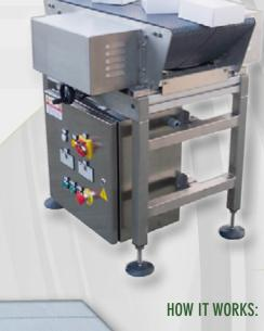
The device is made of a pair of close belts with different speeds that allows to change the product orientation even at high speeds. When the product enters the device, it undergoes an horizontal rotation due to variable speeds. The rotation angle can be controlled acting on the delta speed of the two belts and on the product positioning according to the axis of the device. The main assets are continuous rotation, compactness and easy maintenance in addition to a great versatility.
